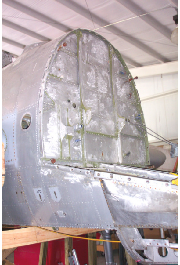
Firewall bead blasting
