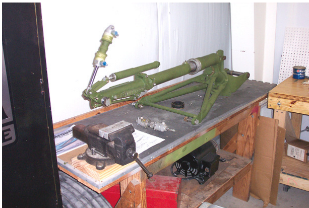
Rebuilt tail wheel assembly
